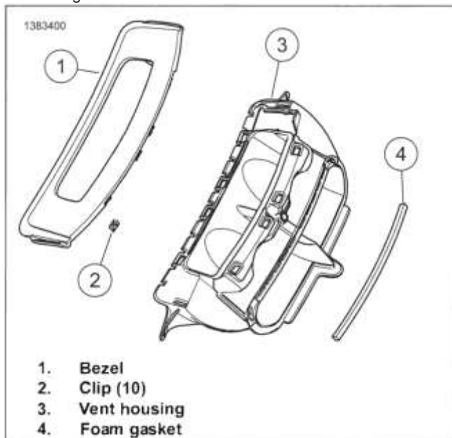
Figure 3-107. Fairing Vent Assembly
