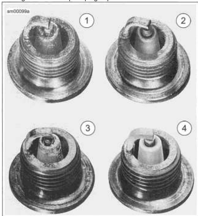
Figure 2-45. Spark Plug Deposits
