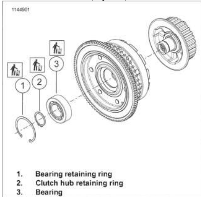
Figure 5-22. Clutch Retaining Rings
