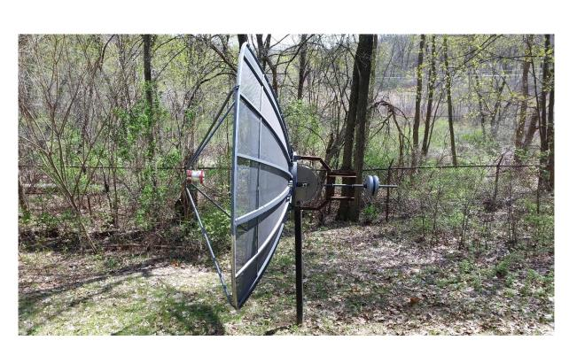
MHAS 3m Dish Antenna, Repurposed from a C-Band Satellite TV Receiving System (1980's Vintage)
