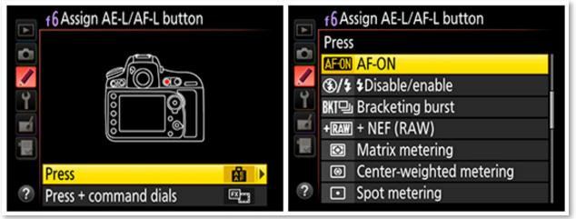
When you press the option to Assign AE-L/AF-L button, you'll have an option for just Press – that's the one you want. On the next menu, select AF-ON and hit the OK button on the back of the camera.
