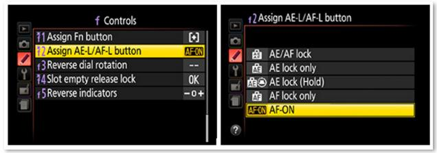
Switching the AE/AF Lock button to AF-On duty on the D6xx and D5xxx series.
