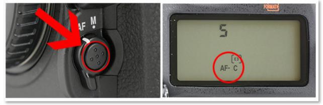
Press and hold the Focus Mode Button as you turn the Main Command Dial on the back of the camera to switch AF Modes.
