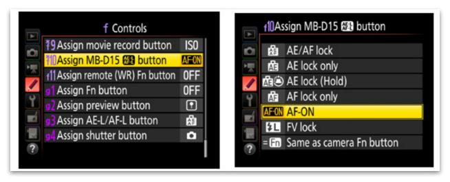
Note - these screen caps are from the D7200, but the procedure is the same for any Nikon camera with a grip featuring an AE/AF-L button. Just note that the number will vary. For instance, on a D7200, it's MB-D15, for a D810, it's MB-D12.
