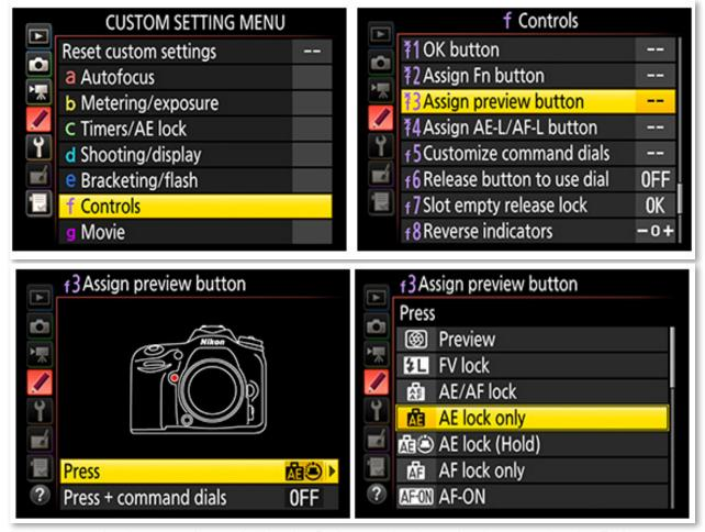
In the example above, we're assigning the Pv button, but it works the same for the Fn button.
