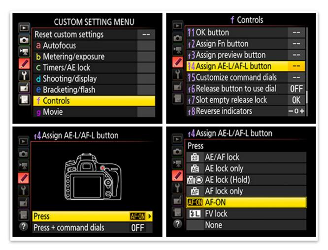
Switching the AE/AF Lock button to AF-On duty on the D750 / D7100.
