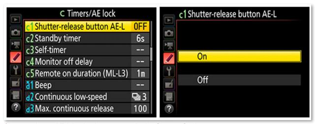
Shutter release AE-L is simple to set up via the Custom Setting menu.
