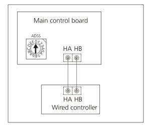
For some models: The wired controller connects to terminal board, terminal board connects to main control board.
