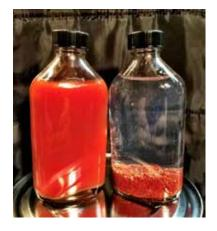
You may add SlurryDry to the remaining thickened sludge material to dehydrate the remaining moisture and creating a safe material for standard disposal that meets the requirements for the EPA 9095B Paint Filter Test for adequate moisture levels. SlurryDry's main ingredient is EPA compliant as an acceptable non-biodegradable sorbent. SlurryDry adds further encapsulation of contaminants and is highly resistant to leaching providing a cost effective method of safe disposal.
