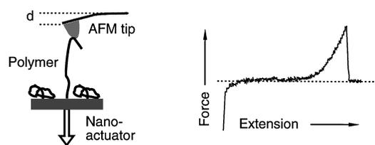
FIG. 1. A typical experiment in which a single molecule is stretched by an AFM tip. The tip is brought into contact with the sample, which is covered by a layer of polymer molecules. If a molecule has bound to the tip it can be stretched and the force is measured via the deflection of the cantilever spring as a function of the extension. When the maximum binding force is exceeded, the molecule ruptures from the tip and the tip is free again.
