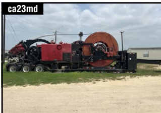
2006 AMKIN DCT150V Stk# 14888, RECONDITIONED 2012, COILED TUBING UNIT 1 1/2" 18,000FT, POW-
