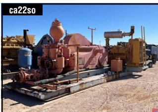
CONTINENTAL EMSCO DB550 DU- PLEX PUMP P/B: V-12 DIESEL EN- GINE W/ PULSATION DAMPENER
