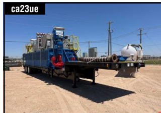
1998 WABASH TRAILER MTD MUD SYSTEM W/ 8'W X 4'H X 23'L 130 BBL OPEN TOP MUD TANK W/
