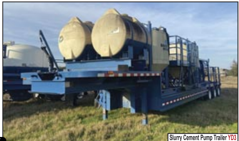
Slurry Cement Pump Trailer YD3
