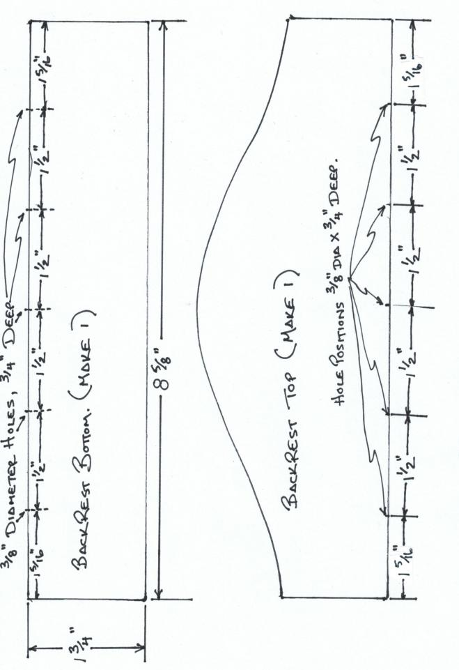
Cut Spes of 38" DIAMETER DOWEL @ 7" LONG EACH.
