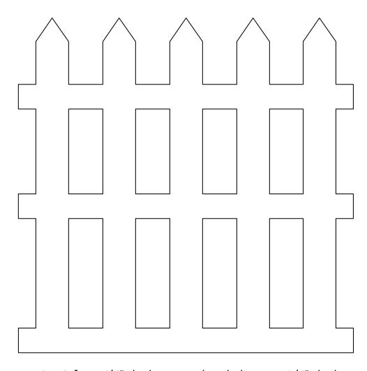
Cut 2 from 1/4" thick material and glue to a 3/4" thick base that measures 5"X1-3/4"
