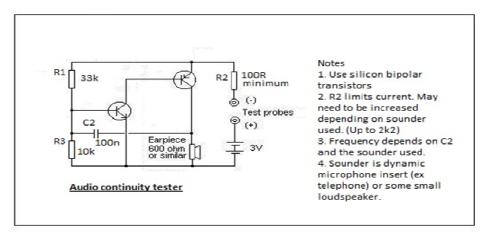
Test for continuity in a circuit A low resistance in a circuit will be detected by a change in tone.
