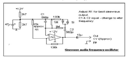
Practically any general purpose Op amp can be used. Next month a tuneable filter will clean up the output although this oscillator output is very good for general use.
