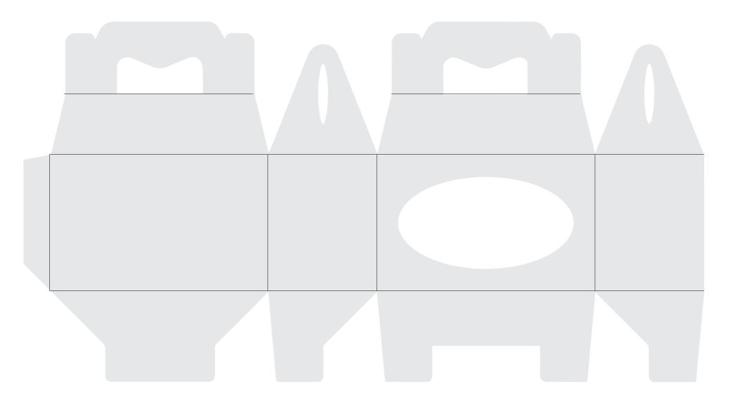
Print scale at 100% / print on the back (white side) of the cardstock / black lines are the score lines (do not cut these)
