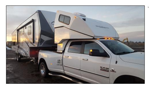
A SWITCH RAISES AND LOWERS THE UNIT TO EASILY ADJUST FOR OPTIMAL WIND DEFLECTION WHILE TOWING, OR FOR SLEEPING - DRIVE IT IN ANY POSITION
