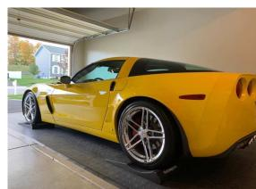
general. The good thing is that as you drive, your tires rotate, obviously, and your tires warm up. Both of these actions will work the "set" out of the nylon cap meaning that the "flat spot" will go away and the vibration will diminish to normal levels. The amount of driving distance and time will vary, but achieving normal highway speeds for over 20 minutes will relax most flat spotting.
