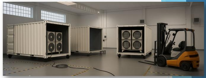
AquaSence is an innovative, self-contained atmospheric water production system designed to tackle the global clean water shortage crisis. Using advanced condensation technology, AquaSence extracts water from the ambient air, purifying it to produce high-quality drinking water suitable for a variety of applications, from humanitarian aid to industrial use.
