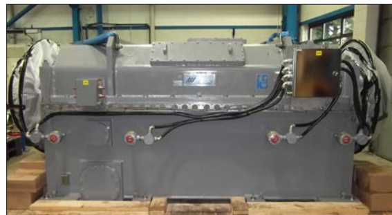
LMS100 Gas Turbine Generator with size 272T SSS® Encased Clutch at Calpine (formerly Conectiv) Cumberland Energy Center, Millville, NJ.
