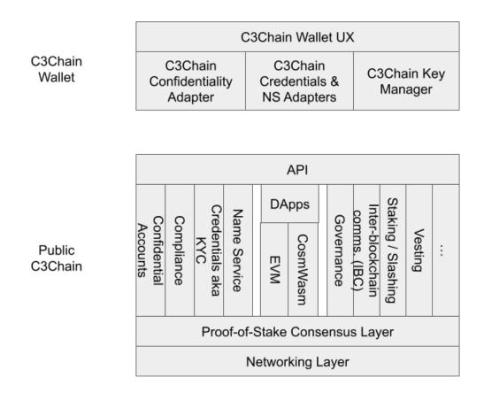
The diagram above shows a high level architecture for C3Q Chain Wallet and the C3Q Chain. Adapters/libraries are provided in both Typescript and Go for the UX to interface with the C3Q Chain.
