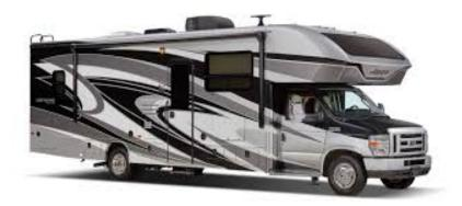
**Super C RV -** The Super C is an RV model that is built on a truck chassis just like a class C. The difference is that the super C is built on a very heavy duty chassis like an International Chassis. Along with the class A RV, the class C is among the most expensive RVs you can purchase. They are able to tow heavy loads and are very roomy inside with slides. They require service at specialized service centers.
