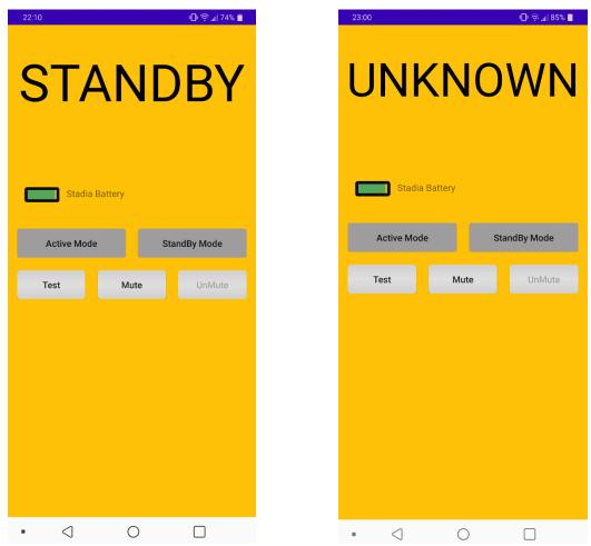
Figure 12 Stadia operation screen displaying "STANDBY" indicates that Stadia is in Standby Mode. "UNKNOWN" indicates that the LIDAR cannot receive clear return signal for measurement
