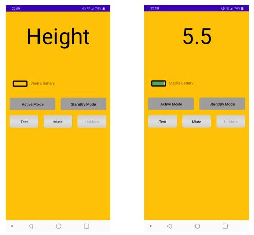
Figure 11 Stadia operation screen displaying "Height" indicating no Bluetooth connection. Screen displaying 5.5 indicates Stadia is 5.5 ft off of the ground
