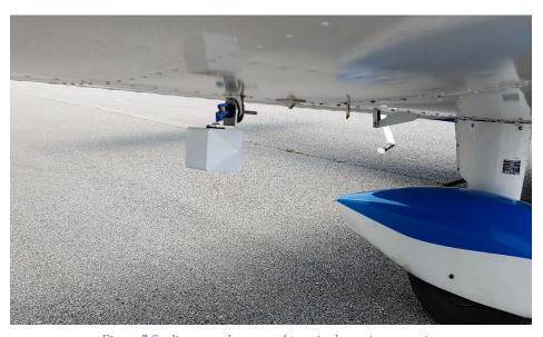
Figure 7 Stadia correctly mounted to a tie-down ring on a wing
