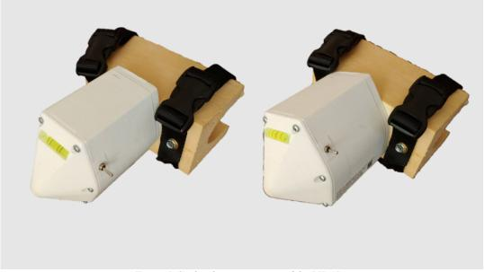
Figure 5 Stadia showing rotation of the LIDAR unit
