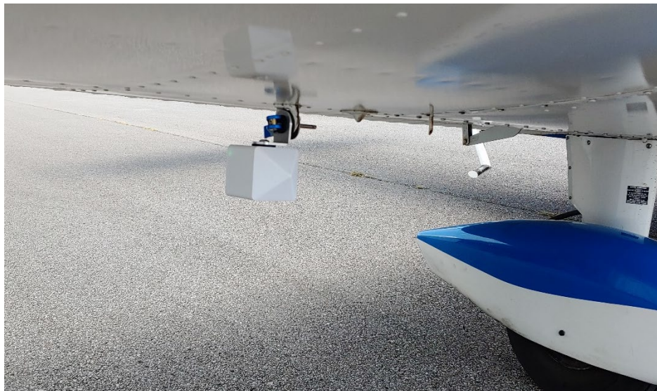
Figure 11 Stadia correctly mounted to a tie-down ring on a wing
