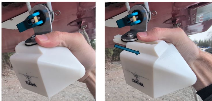
Figure 4 detaching ranging unit on Model L
