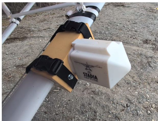
Figure 8 Stadia Neptune showing correct mounting on wing strut
