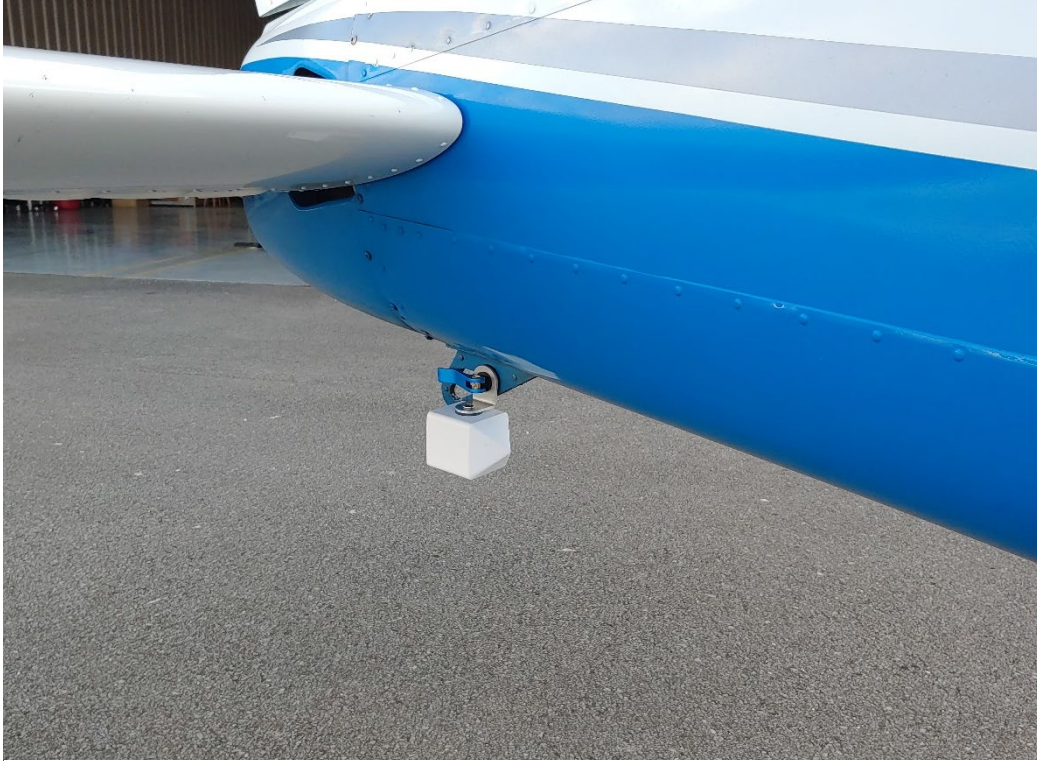
Figure 12 Stadia correctly mounted to a tie-down ring at the tail
