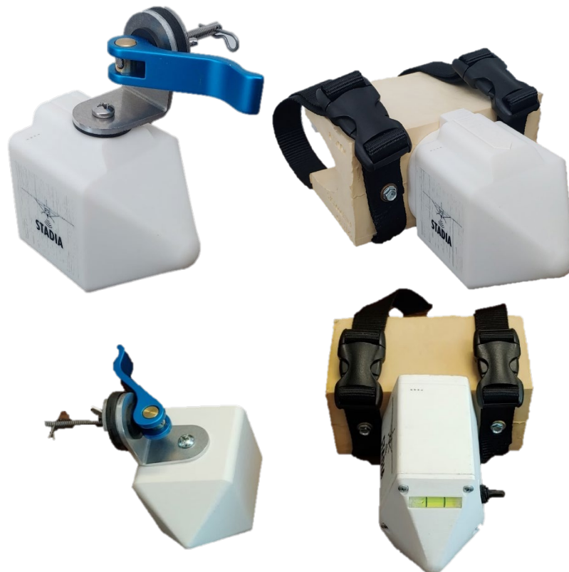
Figure 1 Two models of the 2 nd generation Stadia device above and the 1 st generation below. All units run the same software
