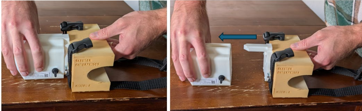
Figure 5 detaching ranging unit on Models A/B
