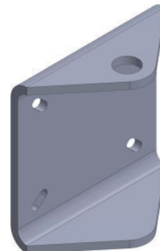
Lower Wall bracket correct installation position
