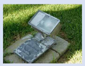
This is an Image of an adjustable spotlight again the damage to the concrete base can be seen, this fixture was also full of water, the Len can also be seen with the same calcium deposits
