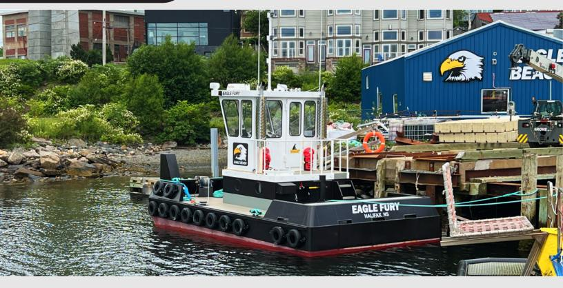
**Eagle Fury** is a heavy duty push boat/ work boat featuring full steel construction. Powered by twin Cummins 305 marine diesel engines with 3:1 gear reduction turning 30" propellors. Up forward she is equipped with a pair of large push knees, two large cleats and 5 ton deck winches making her ideal for manuevering barges and scows.
