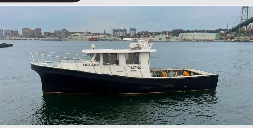
Eagle Leader is a Transport Canada approved passenger vessel/ work boat capable of carrying up to 12 passengers. She has a spacious wheelhouse with seating for 6, with a working galley. Up forward she has 4 bunks along with a fully functioning head as well as a large shower.
