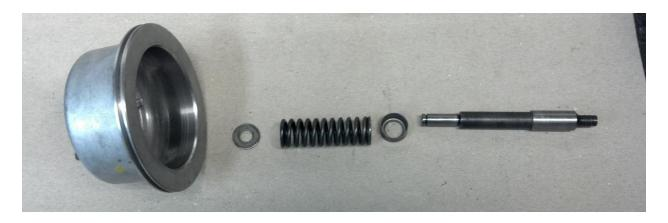
Temporarily assemble the servo apply pin, washer, and servo piston together to check servo/band clearance. You are leaving the spring off to be able to feel the band tension as it clamps the reaction carrier.
