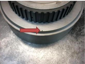
Once all these mods are done, during assembly, install the extra heavy intermediate pressure plate snap ring provided. It may be necessary to sand it with a DA sander or similar to make it fit. Leave the open end or gap at the 3 o'clock position, opposite of the intermediate band anchor for maximum support.
