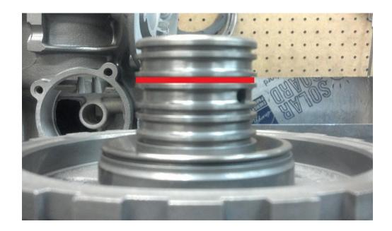
While the direct drum is apart, we recommend using a 1/16" drill bit to drill a bleed hole at the outer edge of the drum to prevent centrifugal apply of the 3<sup>rd</sup> clutches in low gear and also aid in transbrake release if applicable. Take care not to damage the sealing surface.
