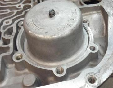
Install 4 checkballs in the case as shown.
