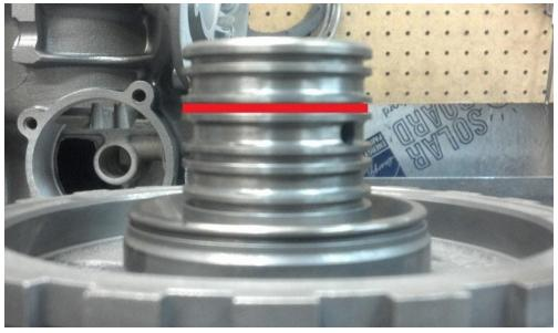
While the direct drum is apart, we recommend using a 1/16" drill bit to drill a bleed hole at the outer edge of the drum to prevent centrifugal apply of the 3<sup>rd</sup> clutches in low gear and also aid in transbrake release if applicable. Take care not to damage the sealing surface. To add the extra clutch and steel provided with the kit you will need to discard the wave plate in the direct drum assembly.
