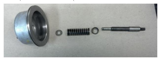
Temporarily assemble the servo apply pin, washer, and servo piston together to check servo/band clearance. You are leaving the spring off to be able to feel the band tension as it clamps the reaction carrier.
