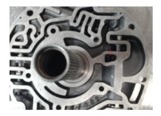
We recommend drilling a .093" hole from the line pressure to the converter charge circuit in the pump as shown. This prevents the converter from suffering charge loss during max line pressure situations.
