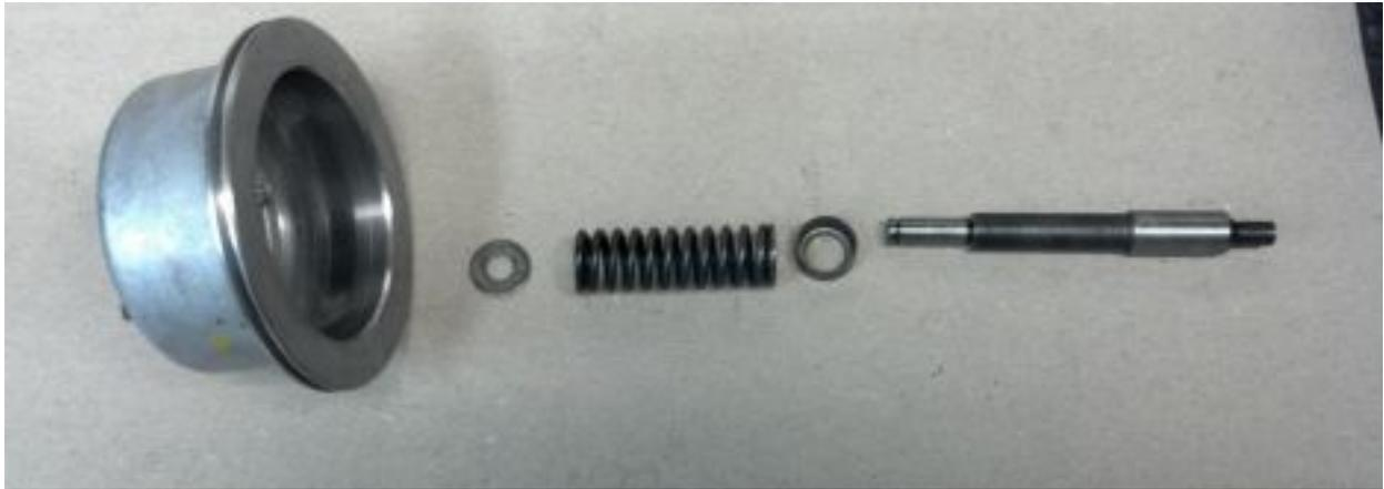
Temporarily assemble the servo apply pin, washer, and servo piston together to check servo/band clearance. You are leaving the spring off to be able to feel the band tension as it clamps the reaction carrier.
