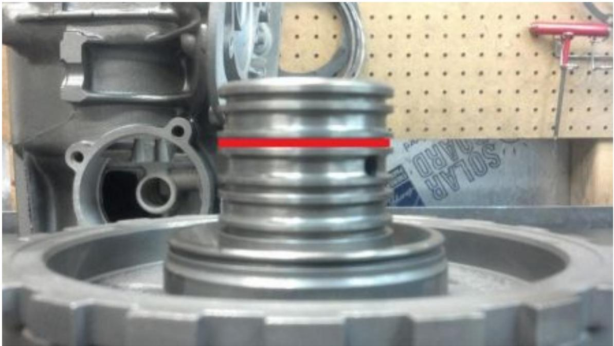
While the direct drum is apart, we recommend using a 1/16" drill bit to drill a bleed hole at the outer edge of the drum to prevent centrifugal apply of the 3<sup>rd</sup> clutches in low gear and also aid in transbrake release if applicable. Take care not to damage the sealing surface. To add the extra clutch and steel provided with the kit you will need to discard the wave plate in the direct drum assembly.
