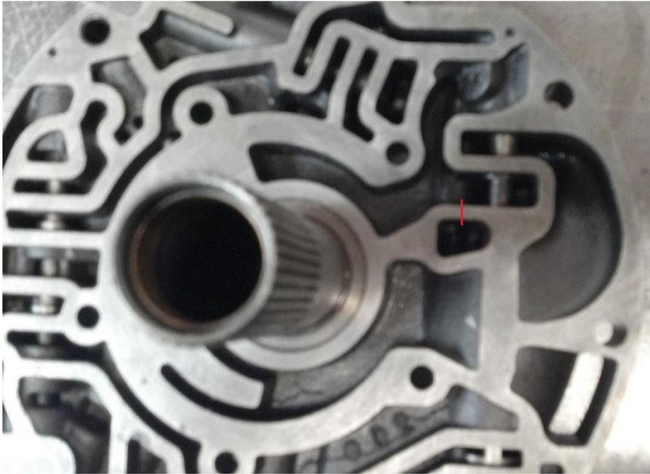
We recommend drilling a .093" hole from the line pressure to the converter charge circuit in the pump as shown. This prevents the converter from suffering charge loss during max line pressure situations.
