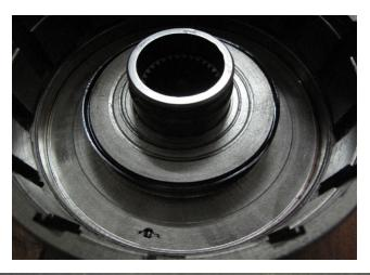
Omit the two seals on the 1-2 accumulator piston (inner piston) shown here.
