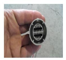
Once this is accomplished, you can poke a hole in the silicone seal using the pick or drill bit, and insert the wires through into the proper location to mate with the wire added to the internal harness.
