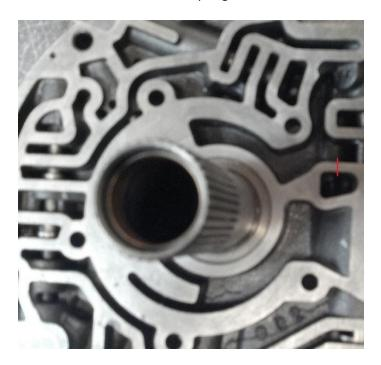
We recommend drilling a .093" hole from the line pressure to converter charge circuit in the pump as shown. This prevents the converter from suffering charge loss during max line pressure situations. The valve body separator plate and accumulator mods have a large part in the shift feel of the unit and also affect long term reliability of hard parts and clutch packs.
