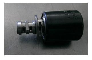
Remove the screens and grind a flat on the middle land of the EPC solenoid as shown. Then install solenoid.
