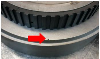
We also leave the center seal off the direct drum as part of the "dual feed" process. The "center" seal seen here on the inside of direct drum should be removed. Also remove the second sealing ring from the front of the center support.
