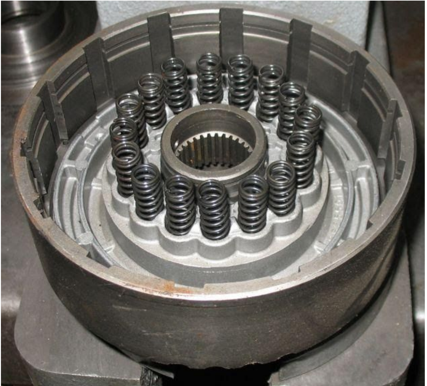
This is a picture of the direct drum with 16 springs, we include 8 Hi Rate springs to replace these. Space accordingly.
