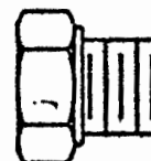
⑫ PLUG, HEX HEAD STRAIGHT THREAD "O" RING
