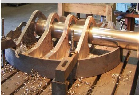
As a result of EIDAL'S need for an extreme duty Fifth Wheel Coupler for its on and off road Heavy Duty Transporters and Load Dividers, EIDAL designed and developed the proven EIDAL Model 1496-1. The EIDAL Model 1496-1 is a heavy duty Rock Lock coupler with a 600,000 lbs pull and 400,000 lbs vertical load capacity designed to oscillate from front to aft.
