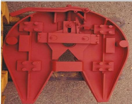
As a result of EIDAL'S need for an extreme duty Fifth Wheel Coupler for its on and off road Heavy Duty Transporters, EIDAL designed and developed the proven EIDAL Model 1167-1. The EIDAL Model 1167-1 is a heavy duty Jaw Type coupler with a 500,000 lbs pull and 250,000 lbs vertical load capacity designed to oscillate from front to aft.
