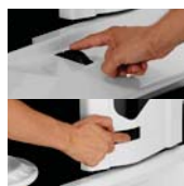
X & Z-Axis Knobs for the Micrometric Movement
