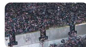
T-Slots Packed with Difficult to Remove Chips
