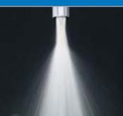
Coolant is Supplied Through Slits of the Tap Holder
