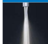
Coolant is Supplied Through Both the Tool and Slits of the Tap Holder
