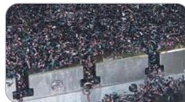
T-slots packed with difficult to remove chips
