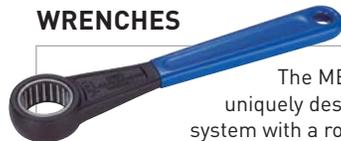
The MEGA WRENCH has a uniquely designed one-way clutch system with a roller bearing and ratchet function that is capable of safely and evenly applying force on the entire nut periphery.
