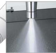
Slit-through coolant with standard MEGA E NUT
