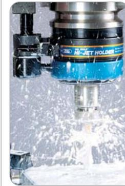
Coolant inducer designed with the bearings in a separate housing from the coolant. This eliminates coolant leakage into the bearings and wear damage to the body, extending the life of the tool.
