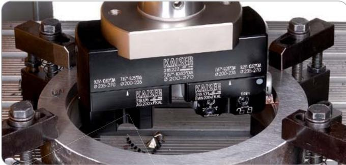
This system is made of lightweight aluminum and can be used for both rough and fine boring, as well as OD turning and grooving applications. It can operate at high speeds of up to 6,600 SFM, and is designed to be completely safe with pinned-to-fit mounting. Additionally, the system comes equipped with coolant supply through all components direct to the cutting edge.
