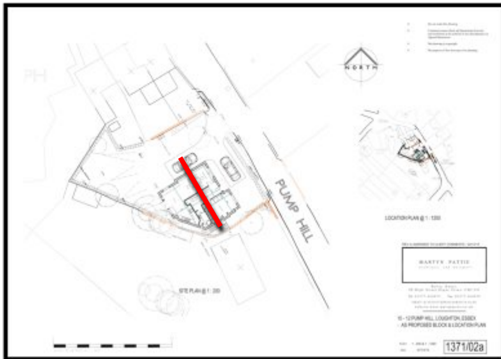
Site plan Area 1 with Trial Trench 1 plotted across central axis of proposed development
