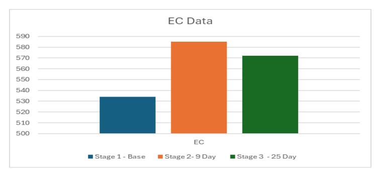
Electrical Conductivity (EC) measures water's ability to conduct electricity, which is directly influenced by the concentration and type of dissolved ions. EC serves as an important indicator of ionic properties, providing insights into the relationship between water composition and system performance. This study monitored EC levels across four distinct phases—Base, 9-Day, 25-Day, and 43-Day (Non-Circulating)—to evaluate the impact of InTenZ on ionic behavior and system stabilization.
