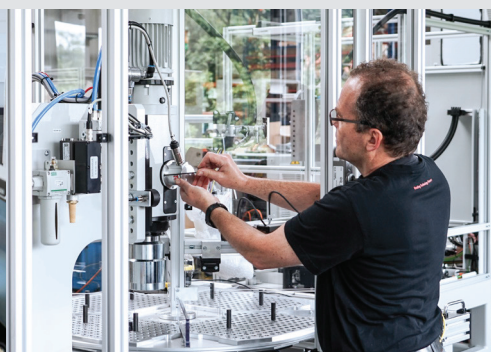
FMW riveting machine assembly in a CNC indexing table machine
