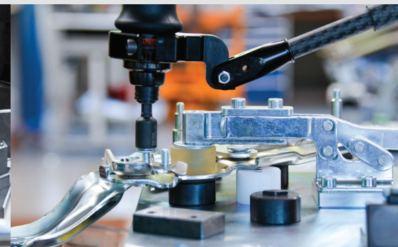
... Bolting station with depth limitation and network interface
