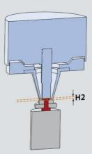
Projection measurement of riveting bolt to the component: Starting with value H1, the riveting process is com- pleted when end value H2 is reached.
