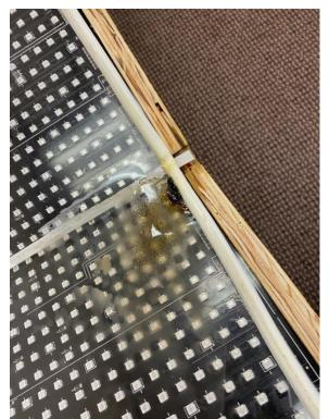
remaining LED circuit boards. A properly designed circuit would not suffer this issue, but this device has no such safety measure. The remaining circuit boards connected to that same power supply leg present a higher temperature which cannot be normalized across the entire surface to the discomfort and potential heat injury of the subsequent device users.
