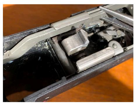
8. Now you need to dislodge the Trigger Bar from the bottom actuator in the rear of the assembly. As shown above. (While holding down the Trigger House Move the Trigger back and forth to have it come loose.)
