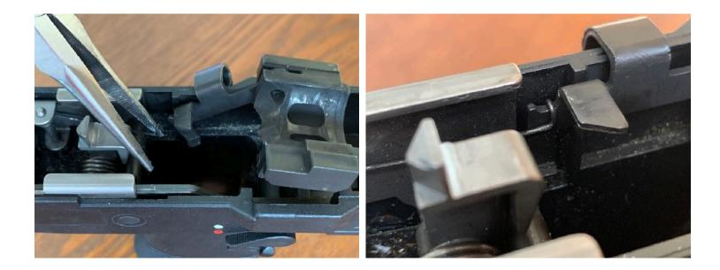
17. Put back the Retaining Clip on the rear PIN
