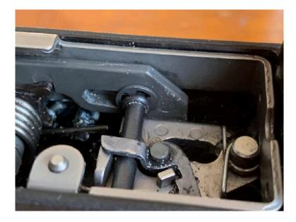
18. Put back the Feed Ramp, make sure to move the Bolt Catch Spring off to the side then once in place back on top.19. Test / Dry Fire Trigger- Test Safety
