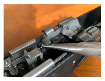
3. Remove the Feed Ramp (pry it up on both sides nothing holds it in place)
