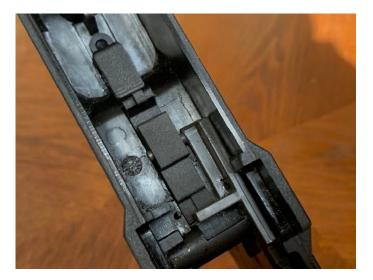
working the trigger in front, while the other helps guid it back into the seat- (It may not move at all you just have to find the right pressure point to use to get it to move and seat).
