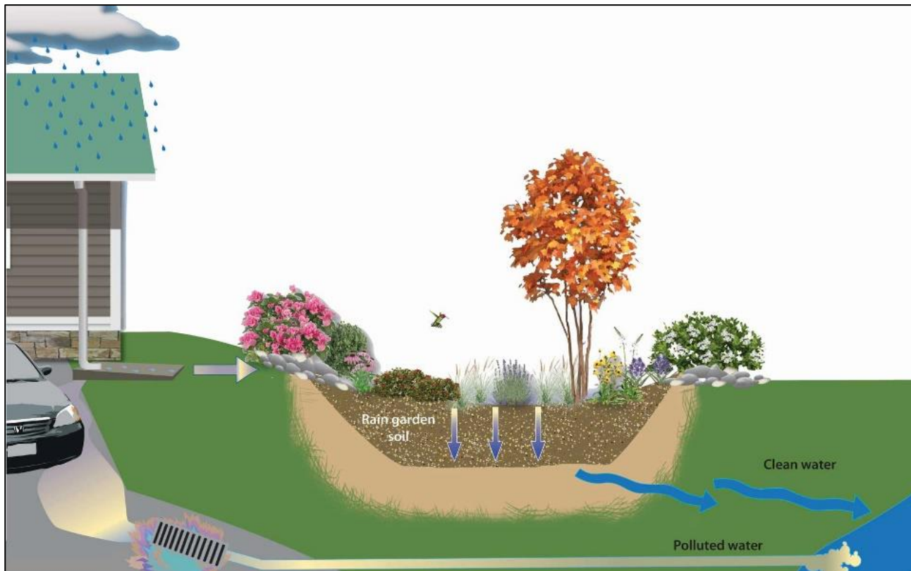
Figure 4. Low Impact Development - Rain Garden Function (Source: Kitsap Conservation District)
