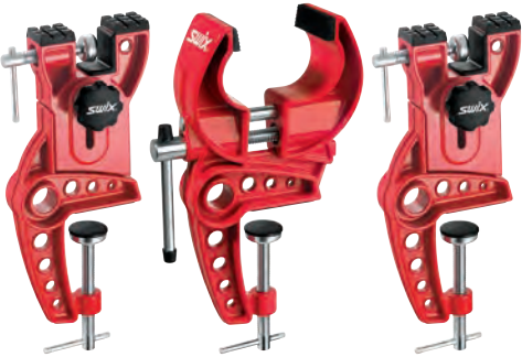
T0149-50 VISE 3-PARTS, 50MM JAWS Swix three piece vise with 50 mm wide jaws. Opens from 40 to 100 mm, for better grip and stability when working on carving skis and radial alpine skis. 60 and 90 degrees side edge working position. Ea.
