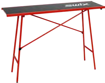
T0075W WAXING TABLE CONSUMER Comes with four rubber feet for anti slip. Adjustable height: 87 cm, 85 cm or 75 cm. One leg adjustable. Table top 120 cm x 35 cm. Fits two sets T0766 Profiles. Net. weight: 11 kg/24 lbs.
