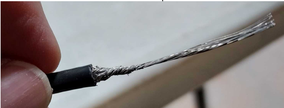
Almost completed termination (non-radio) side of trap, just add solder
