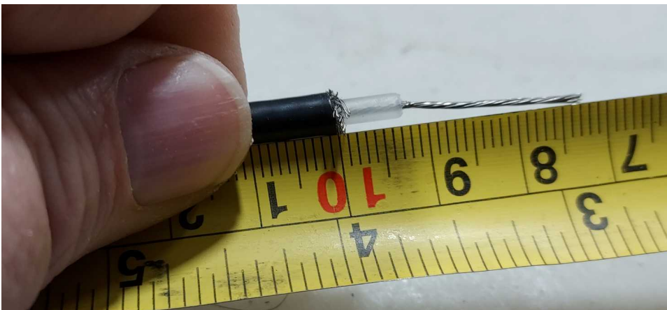
Completed source (radio) side of trap
