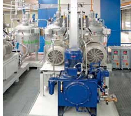
Fully automated high-pressure dosing machine for PUR-foam
