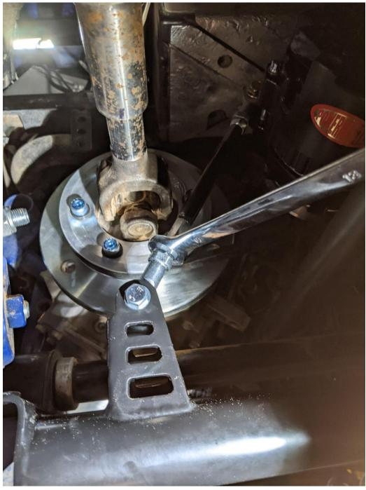
15. Now it is time to install the wiring. Start with the ground, the ends have 2 different sizes: the larger opening is going to the alternator side and the other one goes to the ground on your engine. Reuse 1 bolt (M8x1.25) from the driveshaft flange and install a lock washer and washer on it. This side will be installed on the backside of the alternator wire leading towards the driver side around the alternator bracket, hand tighten the wire for now. Run the other side towards the
