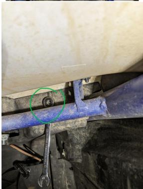
2.9 Once all fasteners have been removed, I found it best to pull on the top right corner and slowly work the firewall out. Be sure to remove the vent line before removing the fire wall.
