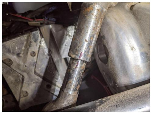
5.3 Now remove the drive shaft by pulling it apart. Now install the pulley with the JTE logo facing the transmission and put the driveshaft back together aligning the marks you put on earlier. **Be sure to install the belt at this point**. Now is a good time to put a small amount of grease in the slip joint although it's not necessary.
