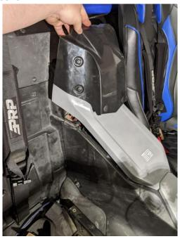
2.3 Remove the passenger side plastic cover. Remove the plastic fastener holding the center trim.
