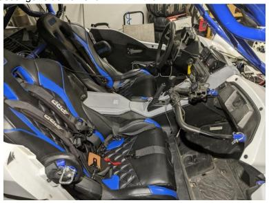
2.1 Remove passenger side seat/mounting bracket using the 12mm socket
