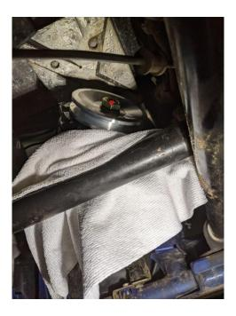
8. Remove the breather and bracket. It is held on with 1 10mm bolt, once removed tuck it out of the way as it's in the way when you install the alternator bracket.
