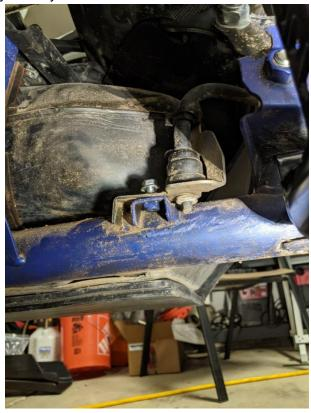
9. Now grab the alternator bracket and install it. Lift the sway bar mounts out of the way to make room for the bracket. Installing the bracket should be nice and easy. When installing the bracket angle the front of the bracket down (Front meaning the part of the bracket furthest to the front of
