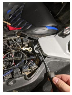
2.4 Gently move the trim up to expose fasteners holding the side cover on.
