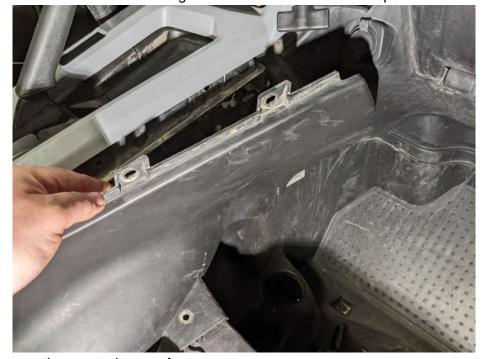
2.7 Now remove the gas tank cover fasteners
