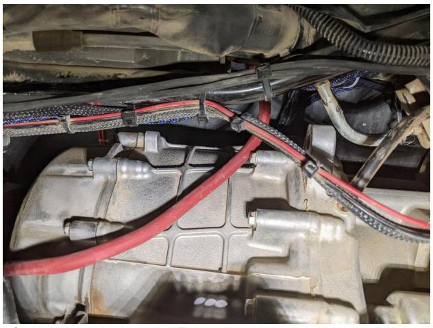
Once cable is routed and connected, Tie it up using cable ties so that it does not rub against transmission, (not shown)
