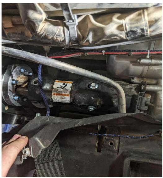
Take the plastic drive shaft shield and reinstall it to the transmission side metal cover. Using the 2 10mm bolts
