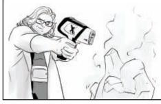
An XRF instrument operates by employing an x-ray beam to excite a sample. As the sample relaxes back to its normal state, it releases a unique secondary fluorescent x-ray. The instrument then detects this fluorescent x-ray to identify the element, and uses the intensity of the energy to quantify the amount of the element present.
