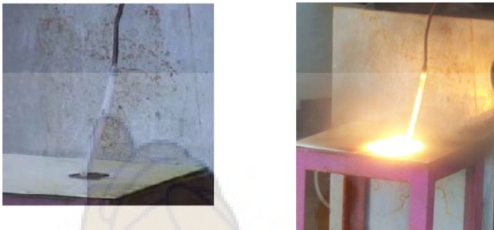
Figure 5: Vapor \text{ClF}_3 Exposure to Polyethylene Tubing, Clean and Used
