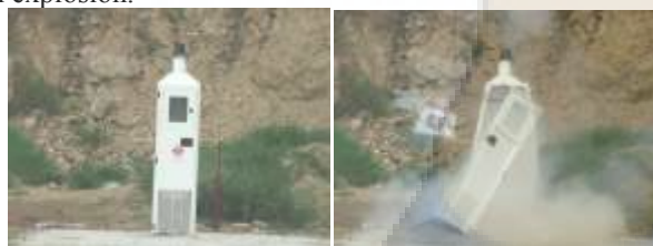
Figure 5. Gas cabinet silane explosion [11] [12] [14] [15]
